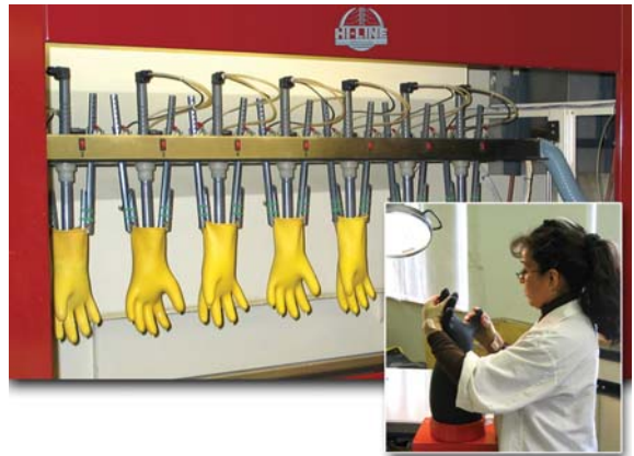
A Hi-Line lab technician runs voltage through a rubber glove to ensure it meets ASTM testing standards.
